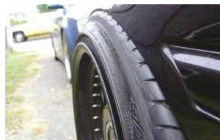
Unsafe fitment of narrow tyres on a wide rim, a case of fashion over sensibility!
