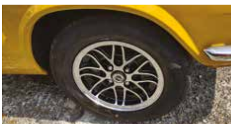
A lot of GT6 owners have fitted larger wheels and tyres, me included as my car has 175/70 13s on 5½J Cosmic Alloy rims.
